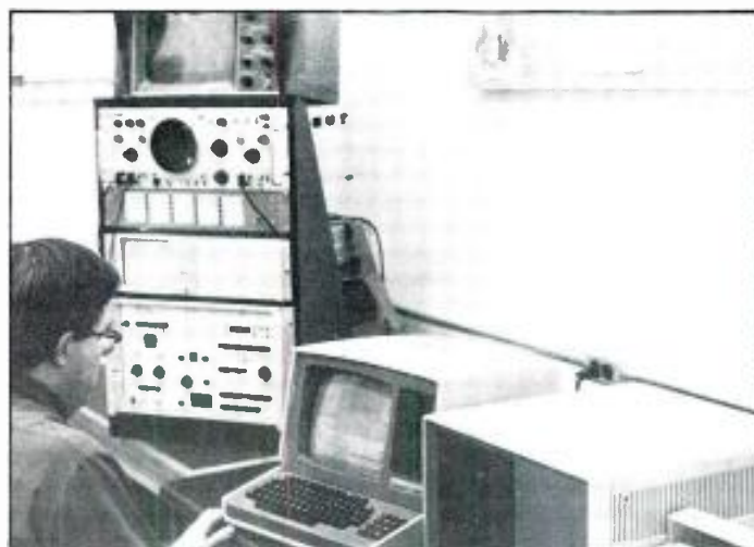
Figure 4. Outputs from the FFT system are compared to determine the difference between two microphones' frequency responses.
